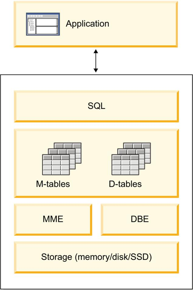
Figure 2. IBM solidDB hybrid server architecture
