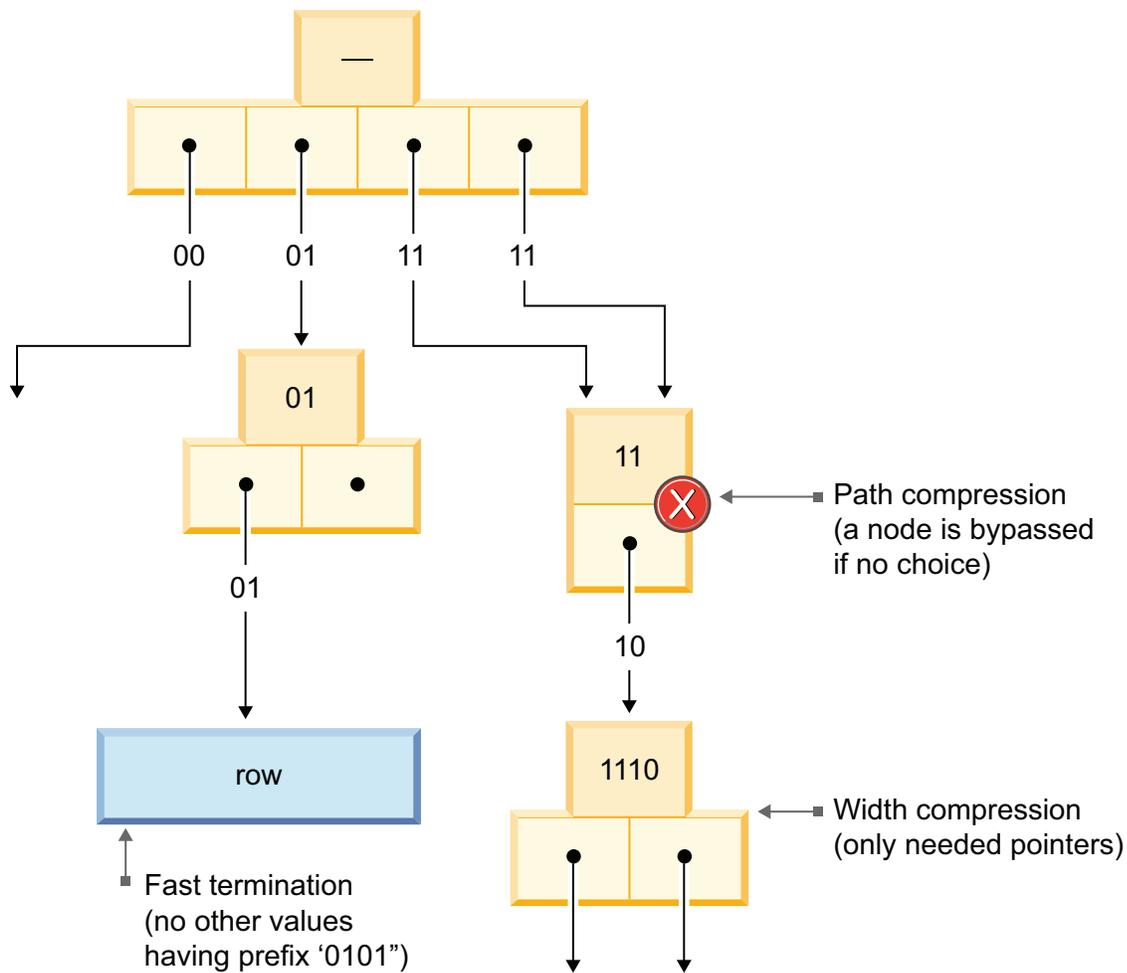
Figure 8. Example of a *VTrie* structure (simplified)
