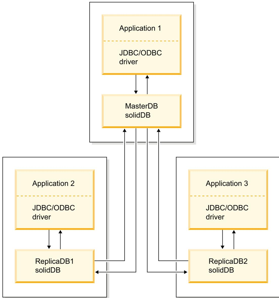
Figure 13. Advance replication installation topology example
